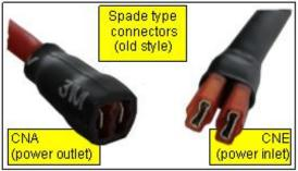
**Figure 1.** Connector types. DT series connectors replace Spade type. Standard configuration: Power lead fitted with DT socket connector and load/receiving side configured with DT pin connector. Polarity: 1 – Black or Gray wire, 2 - White wire.
