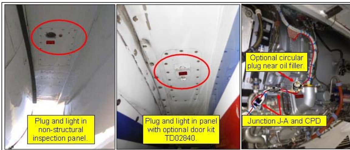
Figure 4.5. Examples for locating plug. Mounting and method TBD by installing authority. Supplied plug and light for flush mounting by voltage, Plug: TP02070-M-115 or TP02839-S-230, Light: TLP3039-115 or TLP3039-230.
