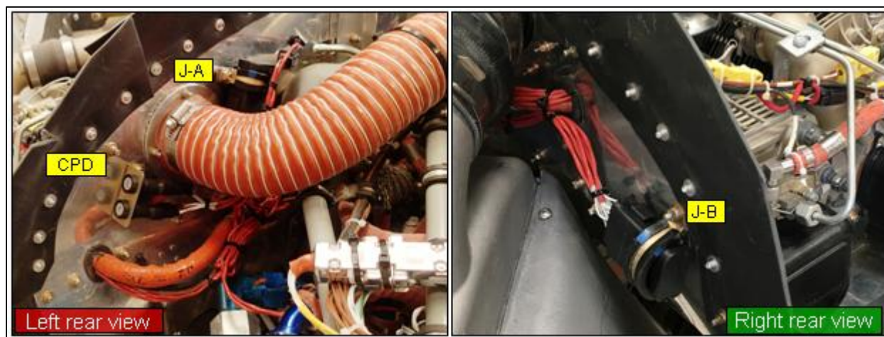
Figure 12 – Locate junctions and CPD (TU03141-B fuse kit) on aft side of engine baffle
