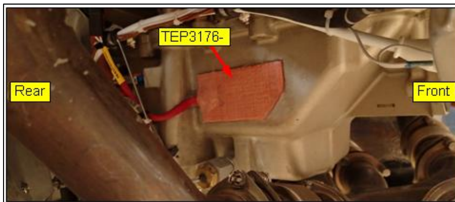
Figure 8 – Oil sump element, locate on right side below nominal oil level lead aft.
