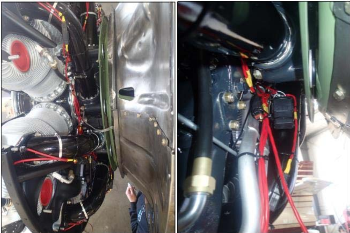
Figure 11 – Examples for locating junctions and lead routing. Locate junctions on aft side of engine, secure with clamps, cable-ties, and/or lacing. Route leads between intake tubes and cylinder bases with ignition leads, individual element leads route on intake tube parallel to primer lines to cylinder head elements, and oil lines to oil tank and cooler elements.
