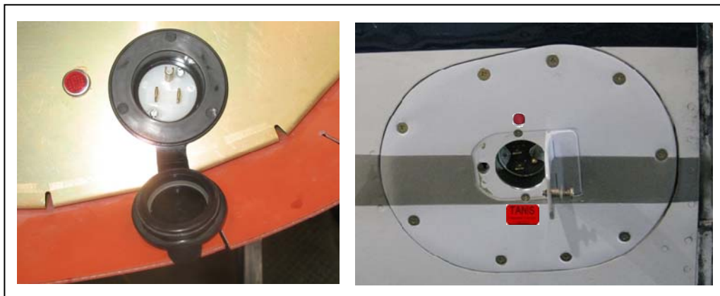
Figure 4-7 Optional shore power plug configurations using flush mount plug, engine baffle, or Tanis door kit.
