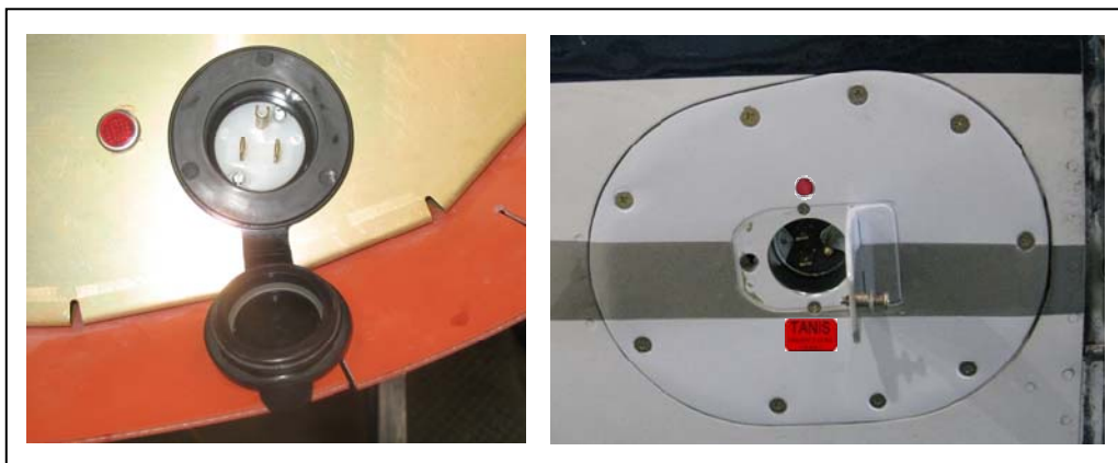
Figure 4-10 Optional shore power plug configurations using flush mount plug, engine baffle, and access panel with Tanis door kit.
