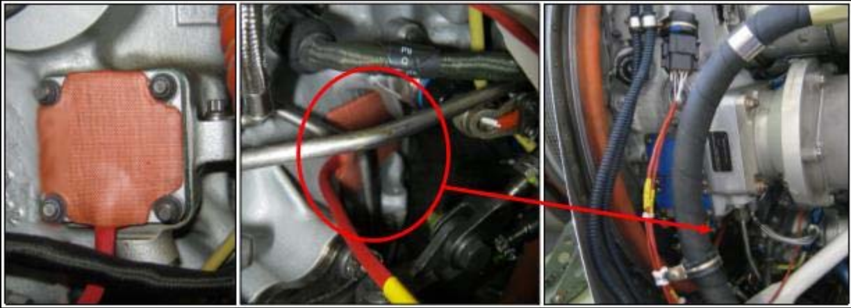
Figure 4. Right engine elements (with AC compressor): Left: TEP3230-, locate on AGB LH cover plate below FCU box. Middle and right: TEP3166-, locate horizontally on AGB RH case below AC compressor.
