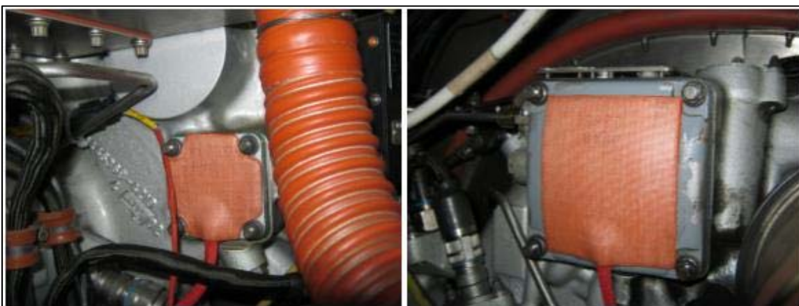
Figure 3. Left engine elements (without AC compressor): Left: TEP3230-, locate on AGB LH cover plate below FCU box. Right: TEP2656-, locate on AGB RH cover plate right of starter generator.
