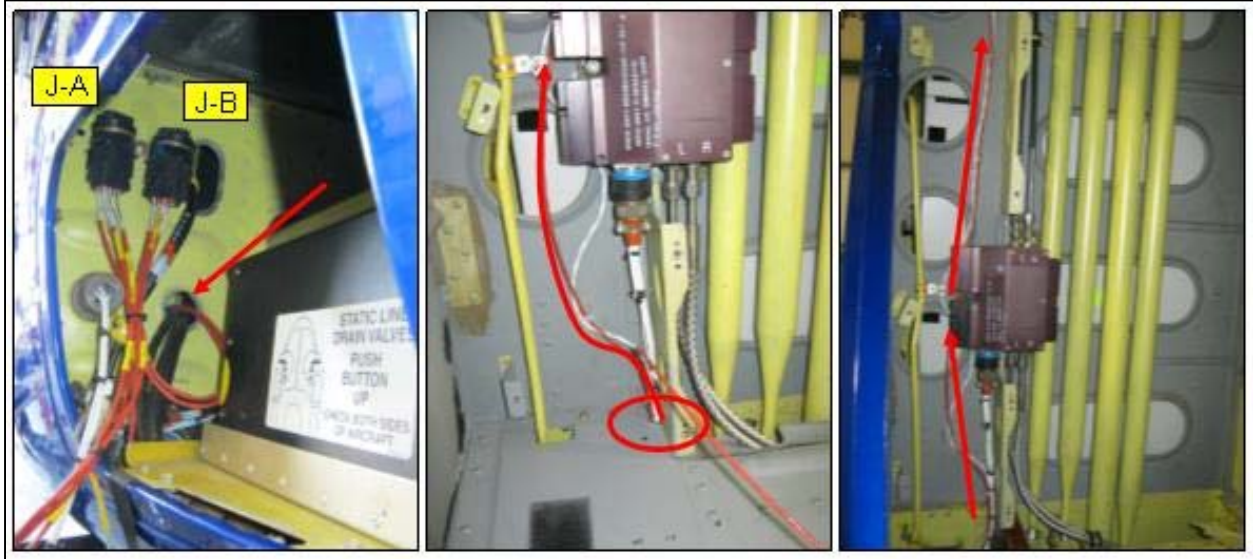
Figure 13. Example of mounting for junctions J-A and J-B and routing from avionics bay aft under floor with engine control cables and existing wiring to upper deck.
