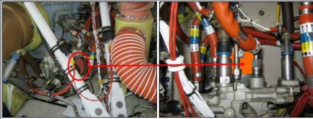
Figure 7. TEP2688-, locate one on each hydraulic unit, low around bottom of circular module.
