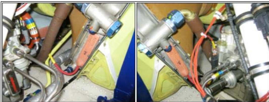
Figure 6. TEP2678-, locate one on each oil cooler below vernatherm valve.
