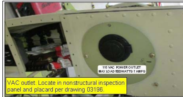
Figure 9. Example VAC plug receptacle (power outlet) installation. Location to be determined by installer, suggest locating in passenger compartment or in aft bulkhead, in non-structural inspection plate. Location varies due to seating configuration, operational requirements, and available space. Placard per cable kit wire diagram 03196 and refer to TN02533.
