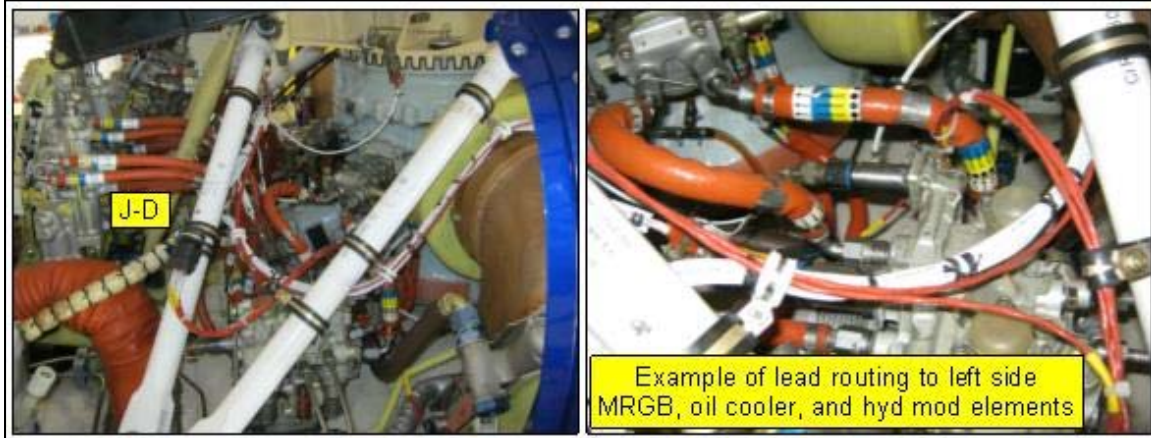
Figure 15. Examples left MRGB junction J-D respective left MRGB truss and leads routed with existing wiring to respective elements.
