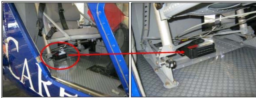
Figure 10. AV/Cabin Heater THP3094-500. Location varies due to seating configuration. Suggest locating as shown, in crew cabin below right front seat with four supplied Click Bond stud mounts CB4000E3CR16 1-inch 10-32 or equivalent CB3000 or 4000 series studs round or trimmed base (-750). Surface preparation: Lightly abrade glossy surfaces with scotch bright or equivalent, to improve the adhesive bond. Just prior to adhesive application, clean surfaces with CB911 solvent wipe, then to prevent redistribution of contaminants dry with a clean dry cloth before solvent evaporates. Do Not use shop towel, rags or paper wipes contaminated with oil, soap, or reclaimed solvents.
