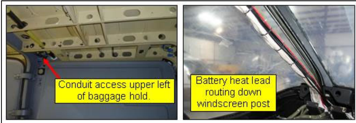
Figure 16 - Left: Conduit access to upper deck for Lead 03. Right: Routing option for battery lead 18 shown down windscreen post, or route lead may be routed with existing wire or battery cables under floor deck.
