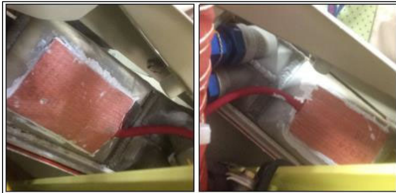
Figure 8B - AW109SP and subsequent with two oil coolers (MRGB oil cooler incorporated with engine oil coolers):
