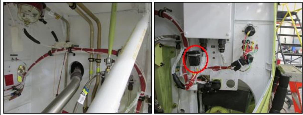
Figure 25 – Junctions J-A1 and J-A2 located with clamps. Use existing spacer and screw (may require longer screw). Junctions located in this area for plug-mounting options A and B. Location may vary due to existing equipment.
