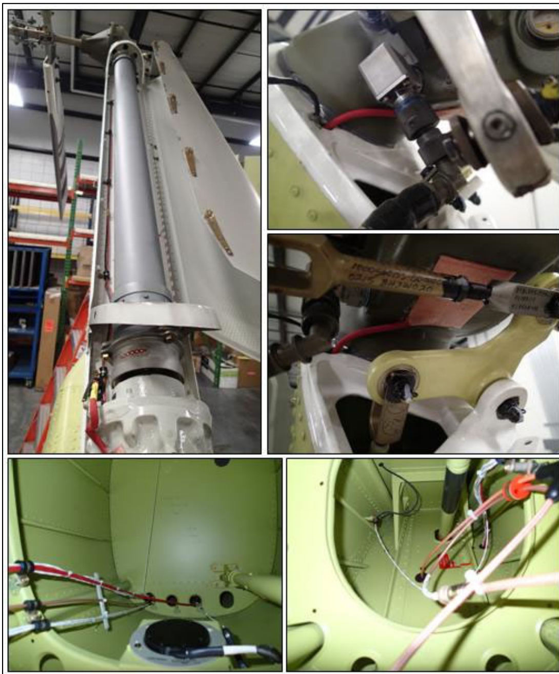
Figure 35 – Example of routing for tailrotor elements, leads 07 and 08. Leads routed together through tailboom disconnect with existing wiring.
