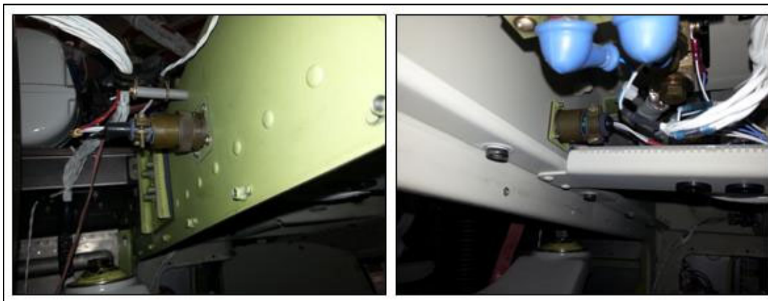
Figure 16 - MRGB connector TU03125 located in upper left or right I beam depending on routing option. Use pre-cut factory holes when available.
