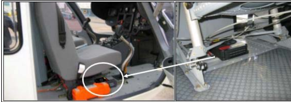
Figure 6.1. Option: Generic example of THP3094 series AV/Cabin Heater (supplied separately). Location TBD by installer, may vary due to seating configuration. Routed into crew cab with existing wiring. For installation and circuit requirements refer to wire diagram 03082, heater operating guide TPG3094 and instructions TN03094.
