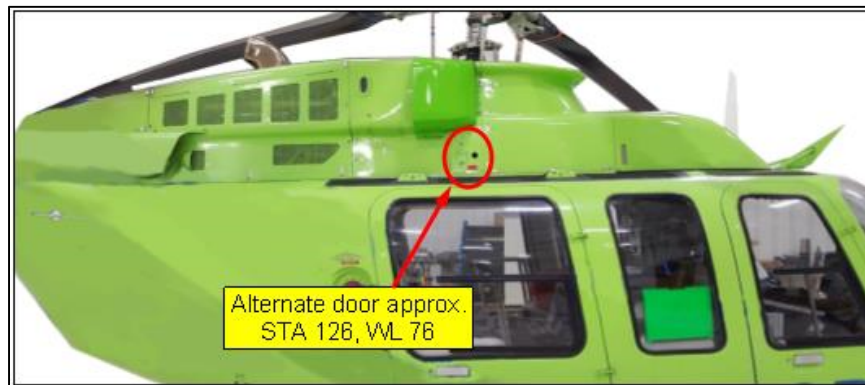
Figure 6.2. Option: Door kit TD02840 (supplied separately). Located in right side of main transmission (MRGB) cowl forward of engine firewall, STA 125, WL 76, approx.
