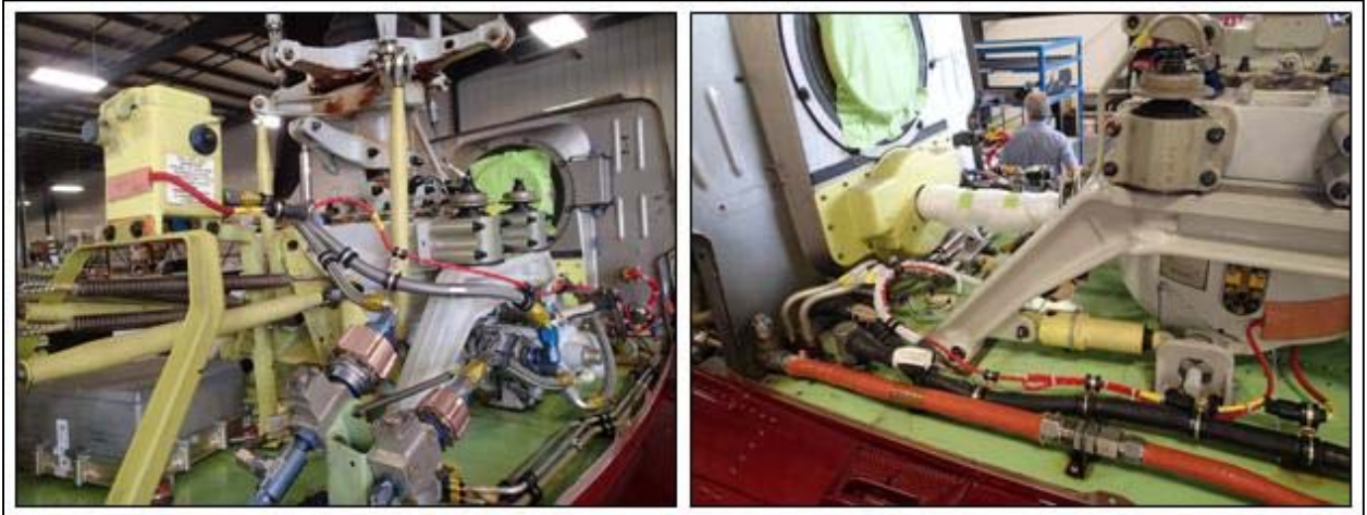
Figure 4.14. Example of MRGB and hydraulic tank cable routing from forward firewall connector and junction J-B.
