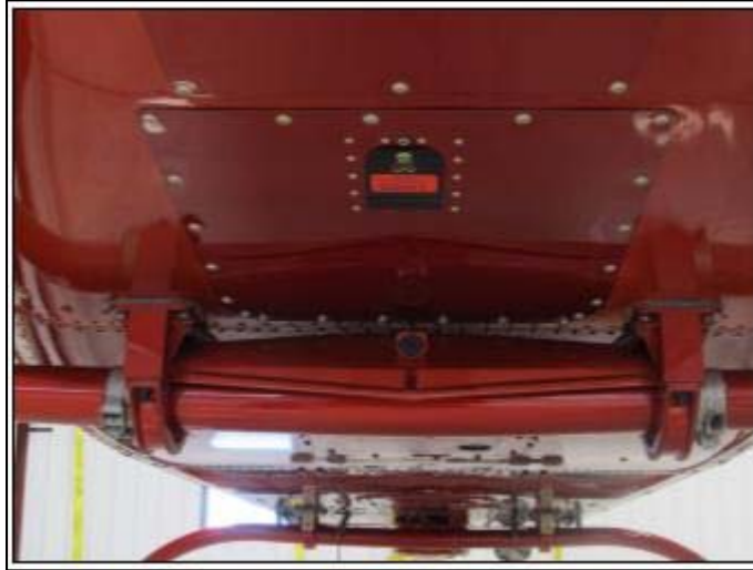
Figure 6.3. Option: Door kit TD02840 (supplied separately) or supplied 2-place door kit. Located in belly panel aft of rear skid near aft edge of panel refer to door kit instruction TN02840 or TN03095 as applicable.
