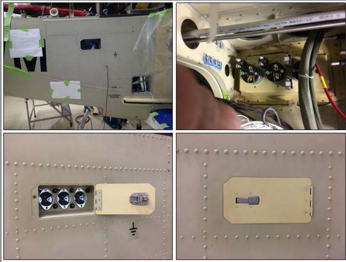
Figure 4.15. Optional Door Kit, field fabricated w/ reference to drawing: 03187 (REF: STA 5210 WL 1006). Uses same plug and placard configuration as Shore Power Kit p/n: TD02935 Figure 4.12.
