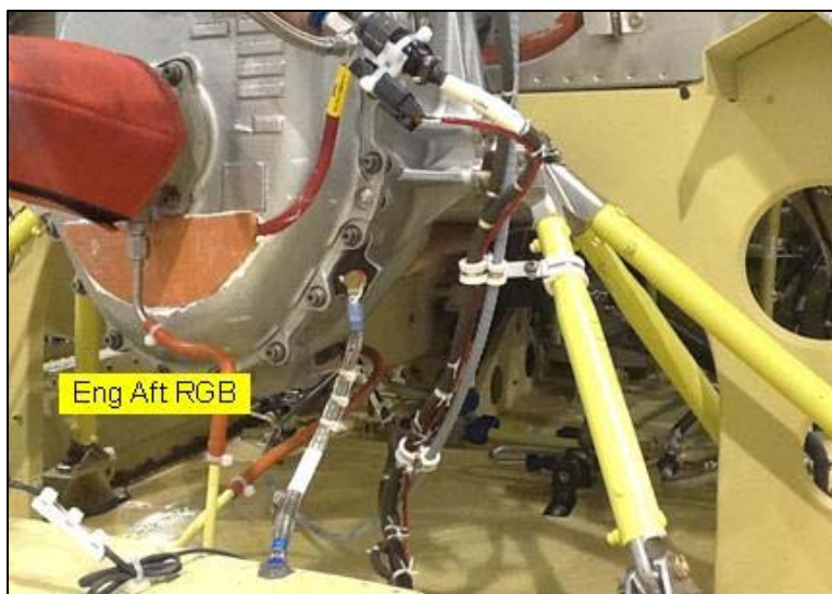
Figure 4.4. Engine RGB Pad Heat Element p/n: TEN2869- Locate on low on case below output lead right to connect w/ lead from J-A.
