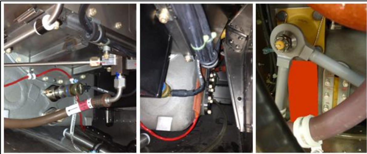
Figure 8 – TEP2675- Each engine oil sump bottom or on right side of sump.
