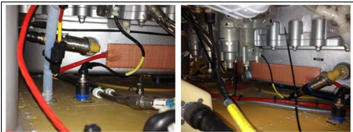
Figure 6 – TEP2650- MRGB front lower sump left and right of center, leads outboard.
