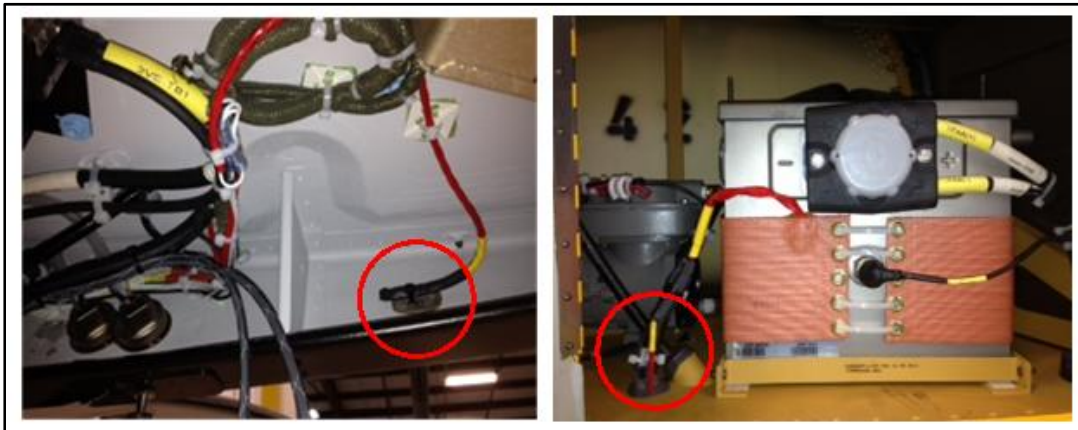
Figure 10 – Battery heat kit supplied separately. Installing cabling and thermal control below battery compartment and route element lead up through deck.
