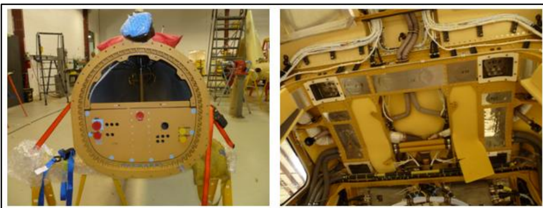
Figure 12 – Left - Routing for TRGB transitions through boom disconnect connector TU03047 installed in boom plate, location varies determined by installer. Right - Option for routing lead between MRGB and Left Engine Junction is along ceiling transitioning through cabin bulkhead, penetrating the main transmission deck with existing wiring or installing Tanis Grommet TG01056 or equivalent. When penetrating composites follow manufactures procedures for potting and edge sealing.
