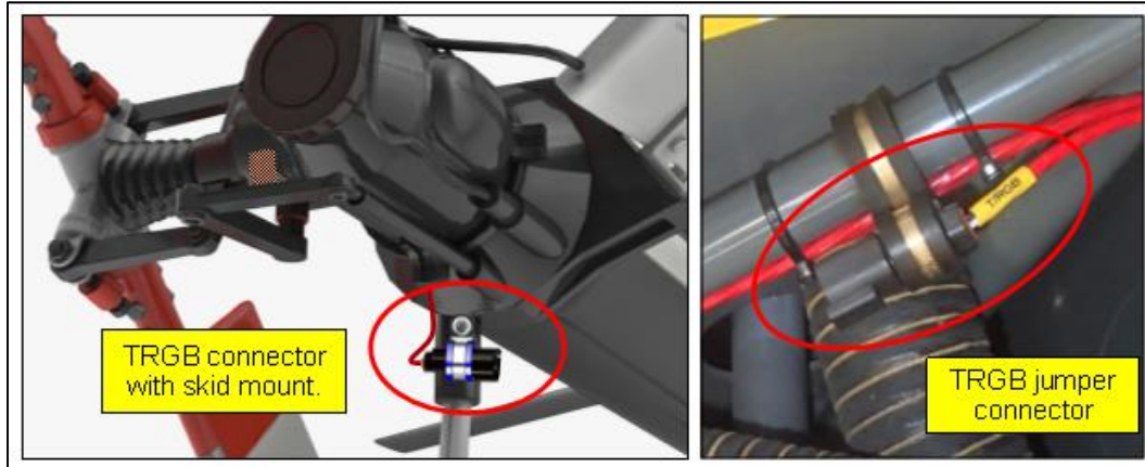
Figure 4.4. Examples of TRGB jumper connectors hard mounted with clamps on airframe.
