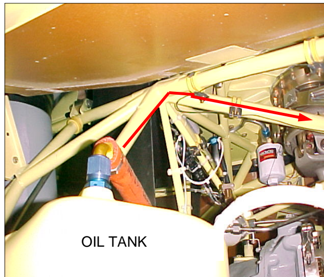
Figure 4-6 Wire routing option from engine to MRGB junction following airframe.
