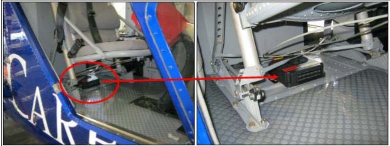
Figure 4.3. THP3094-500 AV/Cabin Heater is to be permanently mounted using supplied Click Bond studs or equivalent. Location TBD and varies due to seating configuration. May be removed for flight or seasonal use. Suggest locating below seat. Power cable from plug routed into crew cab with existing wiring. For additional installation and thermostat options, refer to TN03094.
