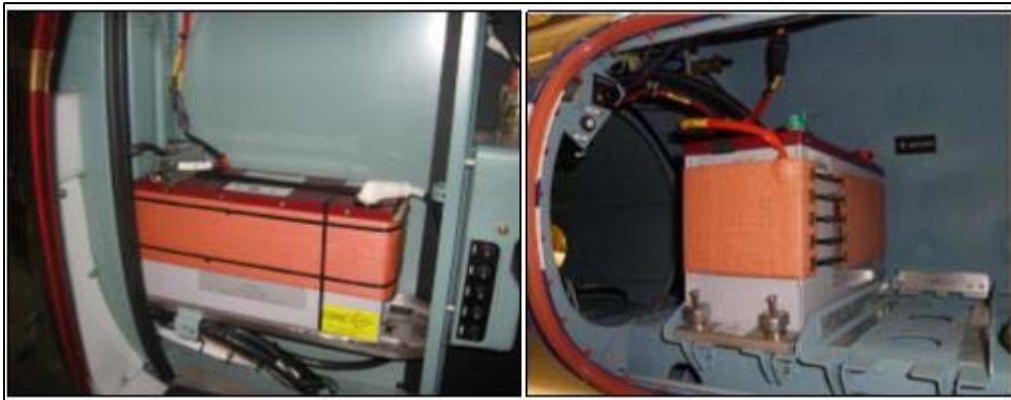
Figure 4.2. TBP2647-31- Battery element (generic example shown, location of battery may vary). Secure around top of battery clear of battery, position clear of bracketing, connectors, and chafe points. Use cable ties or appropriate lacing. Gently lace in place alternating tension between ties. Excessive tension may cause damage or result in pulling grommets through element edge. Note: Due to varying battery configuration and/or location alternate elements available.
