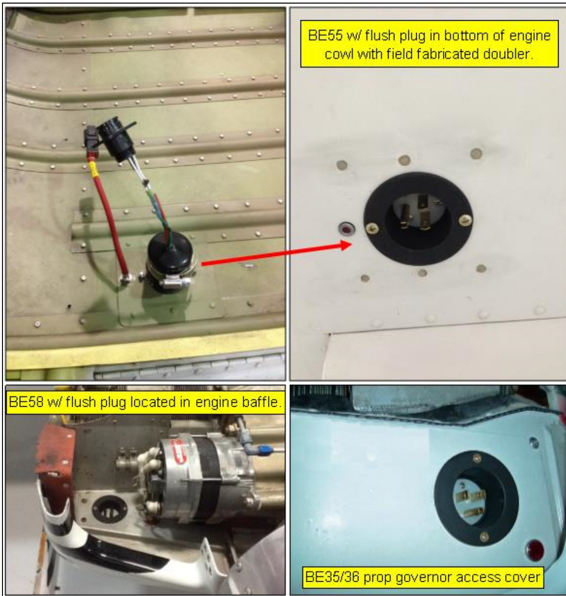
A.6. Examples of flush plugs located on Baron and Bonanza refer to Instruction: TN02070 and TN02533. For additional plug options refer to Appendix §§ B and D.
