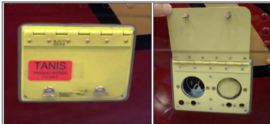
A.14. Example of 2-Place Plug Door Kit p/n: TD03097/TAD03097 located in composite panel. Single plug door kits and cabling options are available, refer to Appendix §§ B and D.
