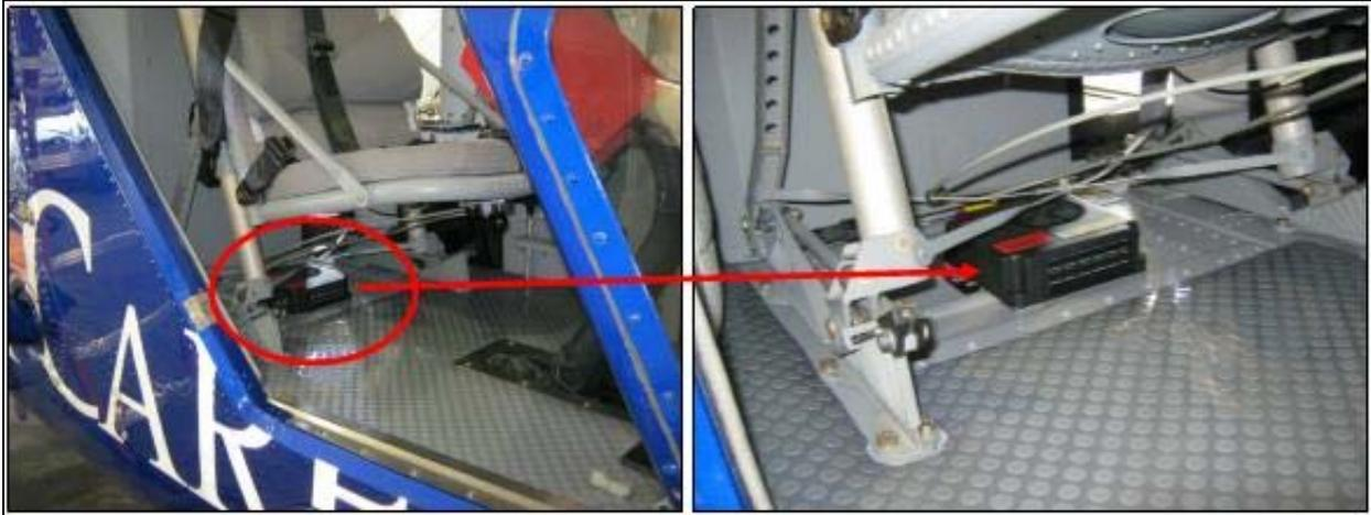
**Figure 7.10.** Example of heater mounted w/ supplied Dual Lock™ Strips p/n: TU03239-02.
