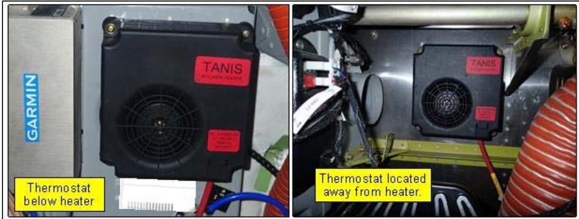
**Figure 7.5.** Examples of AV heater installations.
