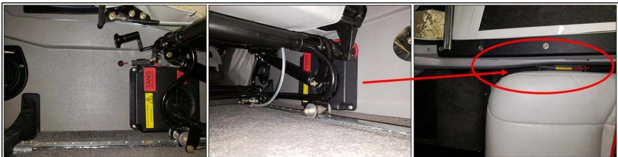
**Figure 7.7.** PA-28 example w/ heater on sidewall below door sill. Installation used existing firewall passthrough for cabling routing from engine preheat power plug. Thermostat remotely located under avionics panel, refer to instruction TN03235.
