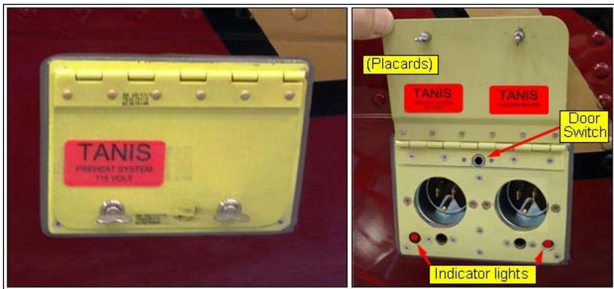
Figure 4.1. Example of installed Door Kit with optional Door Switch. For switch installation refer to Instruction: TN03273.
