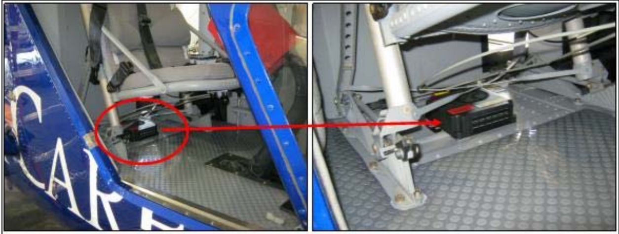
Figure 7.9. Example of heater located horizontally with 1 x 2-inch Dual Lock™ Strips p/n: TU03239-02 (8-each heater).
