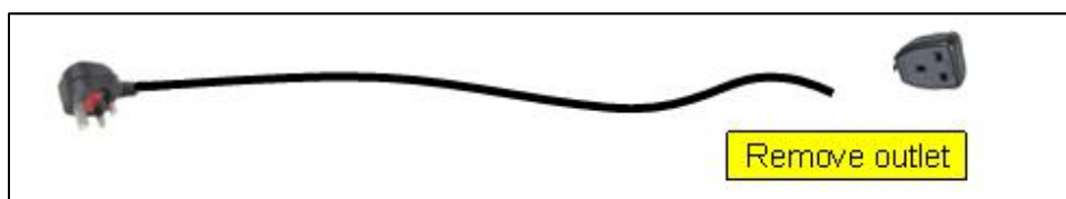
Figure A.2. Preparation: Remove or cut the existing receptacle from the extension cord.
