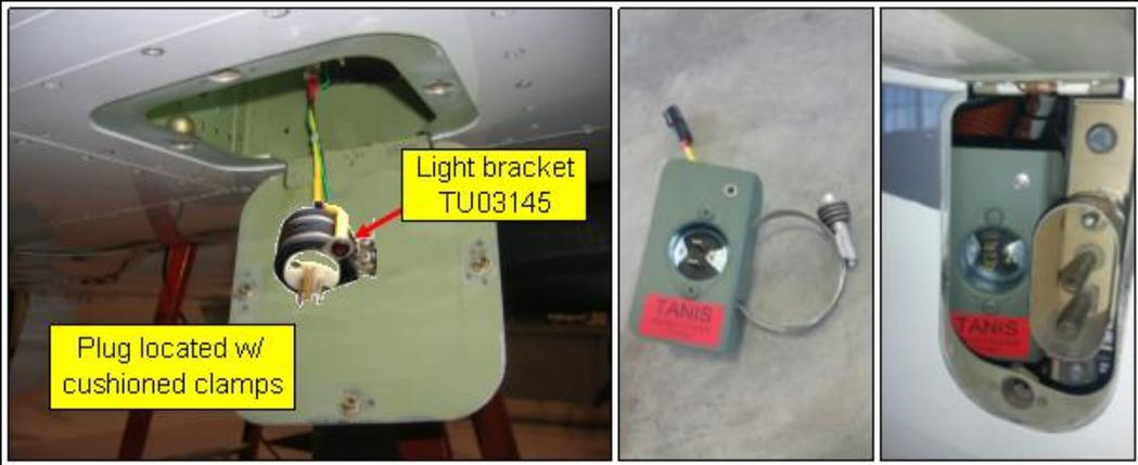
**Figure 4.3.** Examples of plug and light mounting: Plug with clamps, and flush plug mounted in bracket secured to APU connector. For additional plug mounting options refer to Installation Guide TNG1000.
