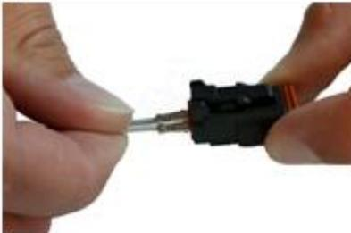
1. Align crimped contact straight into connector seal, per polarity (Note).
