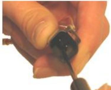
2. Gently pull the contact wire and release the locking finger from the contact with a small screwdriver or pick. See contact diagram page 3.
