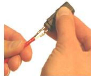
3. Gently pull the contact wire out and then push the seal back in place if displaced.
