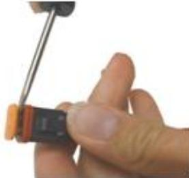
1. Remove orange wedge cap using small screwdriver. Insert between the edge and the body on the narrow side of the connector. Then pull straight out.
