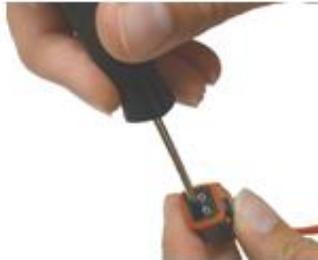
1. Gently pull the contact wire and release the locking finger from the contact with a small screwdriver. See contact diagram page 3.
