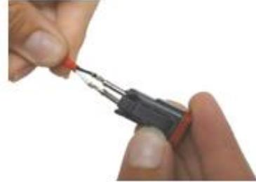
3. Gently pull the contact wire out and push the rear seal back in place if dislodged.
