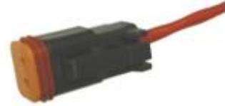
3. Once the contacts are in place, insert a retainer: 2 wire plugs use a wedge/cap with 2 holes. 3 wire plugs use an wedge/cap with 3 holes that the contacts align behind.
