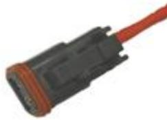
2. Push contact until a click is heard from engagement of internal retention tab. A slight pull will confirm the contact is locked in place.
