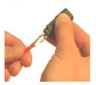
3. Gently pull the contact wire out and then push the seal back in place if displaced.
