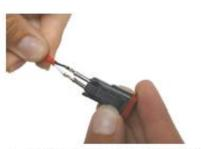
3. Gently pull the contact wire out and push the rear seal back in place if dislodged.
