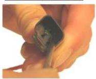
1. Remove wedge using DT-RT1 or seal pick. Pull straight out. For 3 connector receptacles remove the wedge in the middle using pliers.
