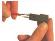
1. Align crimped contact, insert straight into 2. Push contact until a click is heard from connector seal, per polarity ("Note).
