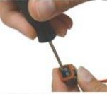
1. Gently pull the contact wire and release the locking finger from the contact with a small screwdriver. See contact diagram page 3.
