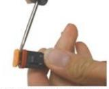
1. Remove orange wedge cap using small screwdriver. Insert between the edge and the body on the narrow side of the connector. Then pull straight out.
