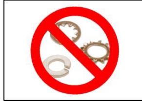
Figure 7.2. DO NOT use split, star, or lock-washer of any type or material. Use of this type of washer will result in element failure.
