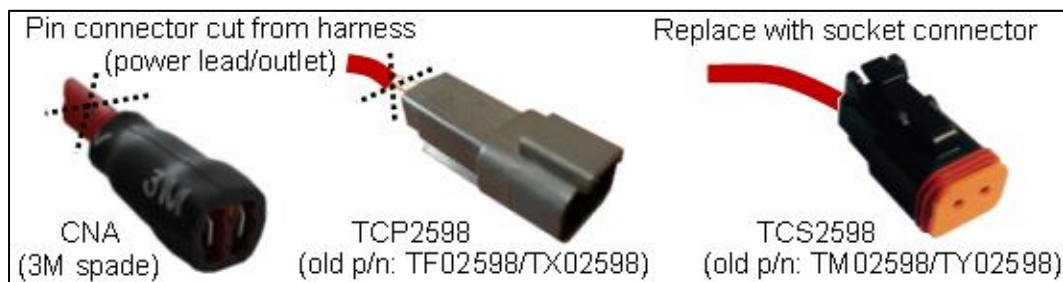
Figure 4.2 Standard electrical configuration assigns concealed socket contacts to connections where voltage or current may cause damage or injury. Element replacement or connector splice may require connector replacement to match standard electrical configuration
