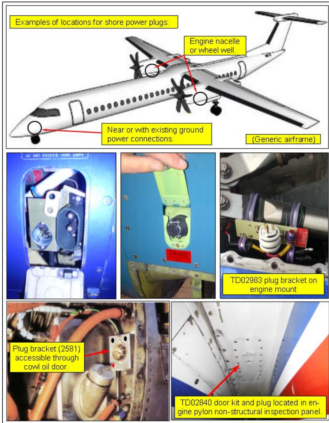
Figure 5. Additional examples of shore power plugs located on airframes.
