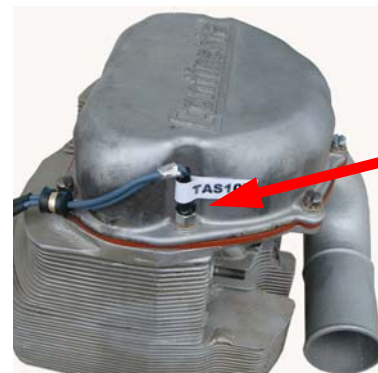
TT02638 on Continental Cylinder with "D" Shaped Cover
